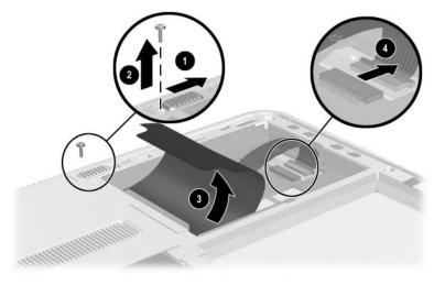
Removing the Display Panel Assembly Screw and Disconnecting the Digitizer Cable
